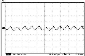
Figure 16: Output voltage ripple, Vout at nominal input voltage and rated load current (10 mV/div). Load capacitance: 1 µF ceramic capacitor and 10 μF tantalum capacitor. Bandwidth: 10 MHz. See Figure 14.
