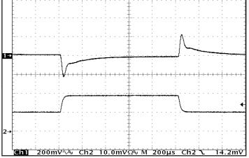
Figure 11: Output voltage response to step-change in load current 50%-100%-50% of Iout (max). Load cap: 1 uF ceramic cap and 10 uF, 100 mohm tantalum cap. CH1: Vout (200 mV/div). CH 2: Iout (10 A/div). Vin=28 V.
