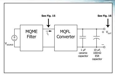
Figure 14: Test set-up diagram showing measurement points for Input Terminal Ripple Current (Figure 15) and Output Voltage Ripple (Figure
