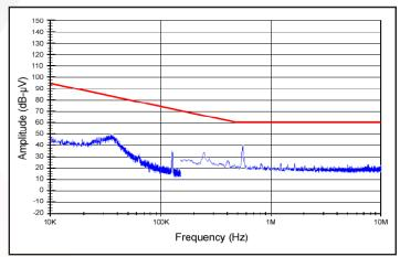
Figure 24: High frequency conducted emissions of MQFL-28-05S, 5 Vout module at 210 W output with MQME-28-P filter; as measured with Method CE102. Limitline shown is the 'Basic Curve' for all applications with a 28 V source.
