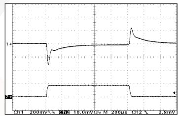
Figure 12: Output voltage response to step-change in load current (0%-50%-0%) of lout (max). Load cap: 1 uF ceramic cap and 10 uF, 100 mW ESR tantalum cap. CH1: Vout (200 mV/div). CH 2: lout (10 A/div). Vin=28 V.
