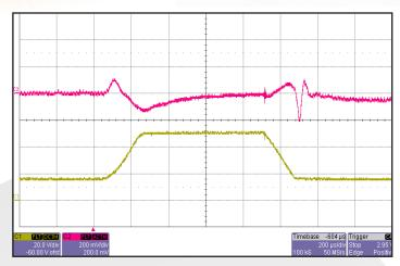
Figure 13: Output voltage response to step-change in input voltage (16 V-50 V-16 V). Load cap: 10  $\mu$ F m $\Omega$  ESR tantalum cap and 1  $\mu$ F ceramic cap. Ch 1: Vin (20 V/div). Ch 2: Vout (200 mV/div).
