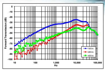
Figure 20: Magnitude of incremental forward transmission (FT = vout/vin) for minimum, nominal, and maximum input voltage at full rated
